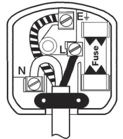
As the colours of the wires may not correspond with the markings in your plug, proceed as follows: The wire which is coloured blue, must be connected to the terminal marked with N or coloured black. The wire which is coloured brown, must be connected to the terminal, which is marked L or coloured red. The wire which is coloured yellow / green should be connected to the terminal which is coloured the same or marked
