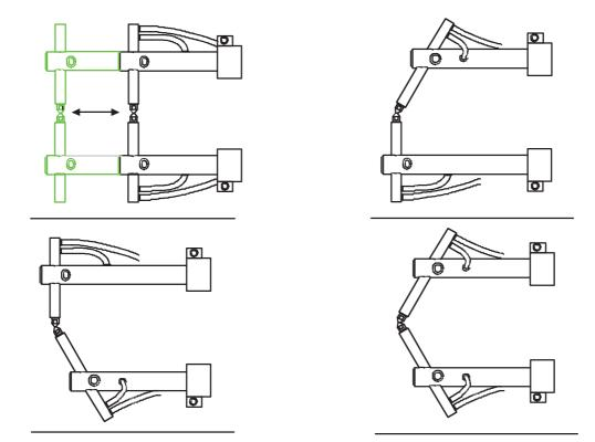
The positions of arms and electrodes can be modified according to the shape of the welding piece:
