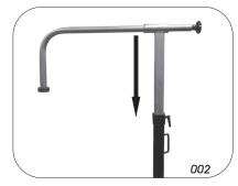
⇒ Slide the roller table shaft slightly through the fixed bracket on the inside of the frame, then place the roller table between the two fixed brackets, slide the roller table shaft through the rear of the roller table and then through the other fixed bracket, secure by using one r-clip, repeat for the other side of the frame (003 & 004).
